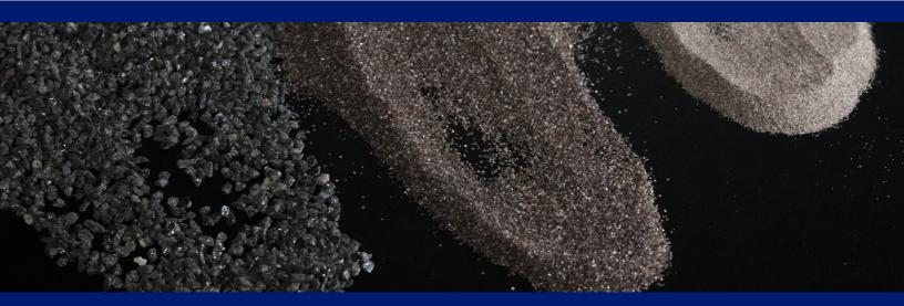
**RockRidge** Aluminum Oxide is manufactured in an electric arc furnace that produces an extremely tough, long-lasting abrasive grain which is graded to macrogrit exacting standards. Aluminum Oxide can be repeatedly recirculated. It is also chemically stable.
